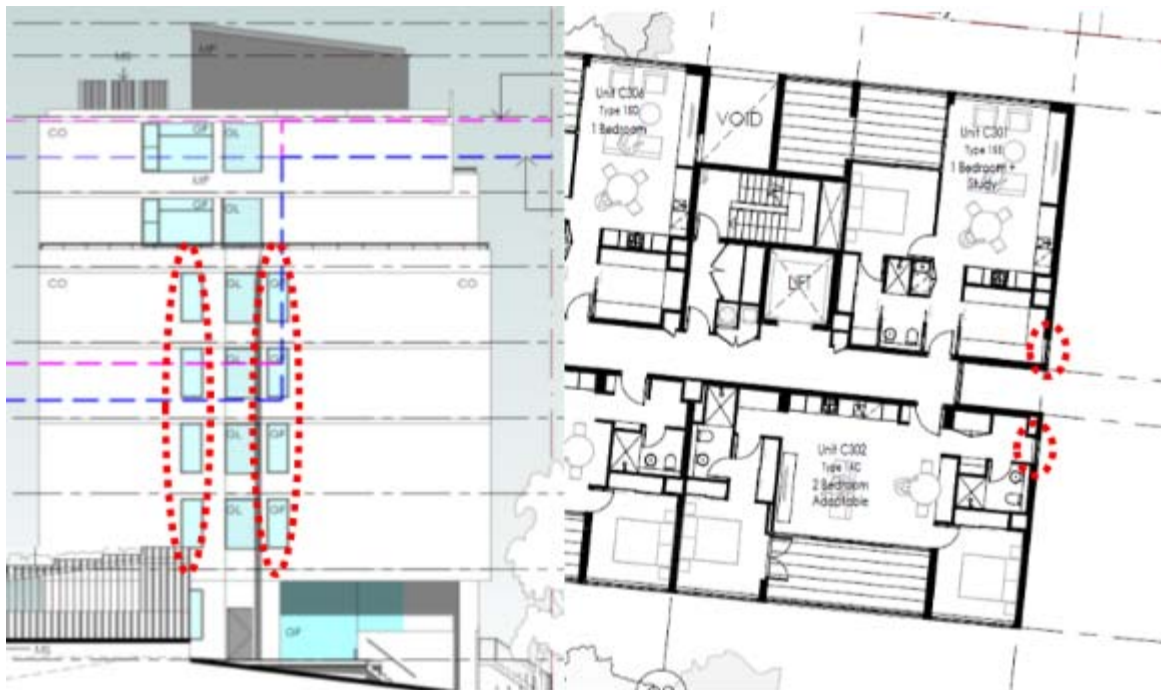
Figure 16: Windows on south elevation of the Hadfields Street building
